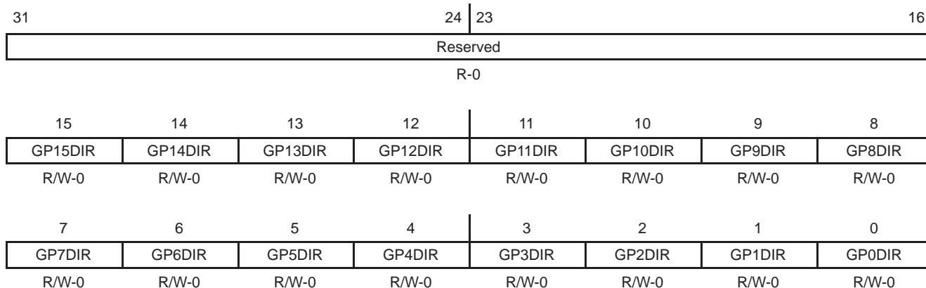
Figure 19. GPIO Direction Register (GPDIR) [Hex Address: 01B0 0004]
