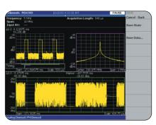
Time-correlated multi-domain view provides a new level of insight about design or operational problems and possible solutions. This example includes frequency, time, and modulation domain views of an AM-modulated pulsed signal with pulseto-pulse phase variation measured in the modulation domain.
