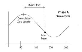
Before phase initialization has occurred the phase offset register will have a value of ffff (hex). Once phase initialization has occurred and the motor has been rotated such that at least one index pulse has been
