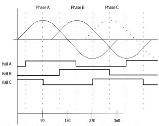
Unlike the algorithmic method, using Hall-based phase initialization no special motor procedures are required. Initialization is performed using the command INIT\_PHASE, and occurs immediately, without any motor motion.
