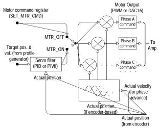
The commutation portion of the chipset uses as input the motor command signal from either the servo filter, or the motor command register (depending on whether the chipset is in closed loop or open loop mode). This pre-commutated command signal is then multiplied by commutation values derived from an internal lookup Sin/Cos table.
