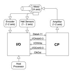
The CP and I/O chips function together as one integrated motion processor. The major components connected to the chip set are the Encoder (2, or 1 axes), (optionally) the motor Hall-sensors (2 or 1 axes), the motor amplifier (2, or 1 axes), and the host processor.
