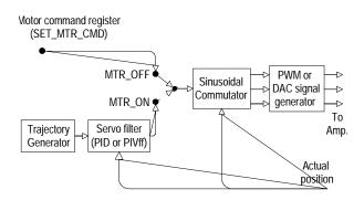
The chipset can be run in either closed loop mode, or open loop mode. In closed loop mode the motor command is determined by the output of the servo filter, which in turn is determined by the output of the trajectory generator and the actual axis position. Closed loop mode is the normal operating mode of the chipset.
