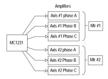
In this configuration the chipset outputs 3 phased PWM magnitude signals per axis. These signals are then fed directly into 3 half-bridge type voltage amplifiers.
