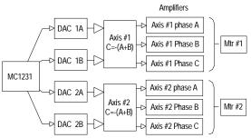
When using DAC output mode the digital word provided by the chipset must first be converted into a voltage using an external DAC. Two DAC channels are required per axis. To construct the third phase for a brushless motor (C phase) the sum of the A and B signals must be 'negated' using C = -(A+B).
