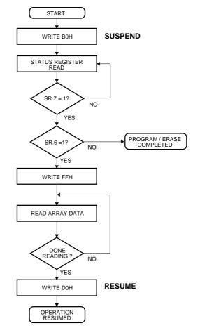
\* The bank address is required when writing this command. Also, there is no need to suspend the erase or program operation when reading data from the other bank. Please use BGO function.
