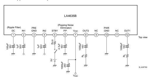
\* If voltage is to be applied to the Standby pin (pin 5), a resistor (Rx) should be inserted to limit the inflow current, as required. Please refer to the information below.
