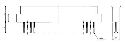
• Recommended board thickness: 0.4 to 0.5mm
