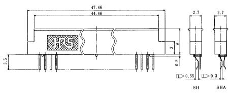
• Recommended board thickness: 0.4 to 0.5mm
