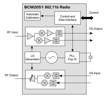
The **BCM2051** 802.11b zero IF Radio is an integrated transceiver device that has been optimized for use in 2.4-GHz 802.11b wireless systems. It has been designed to provide low-power, low-cost, and robust communications for applications operating in the globally available 2.4-GHz unlicensed ISM band. It is fully compliant with the 802.11b specification and meets or exceeds the requirements where appropriate to provide the highest communication link quality of service.
