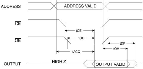
Notes: 1.  $\overline{\text{CE}}$  may be delayed up to t<sub>ACC</sub> - t<sub>CE</sub> after the address transition without impact on t<sub>ACC</sub>.
