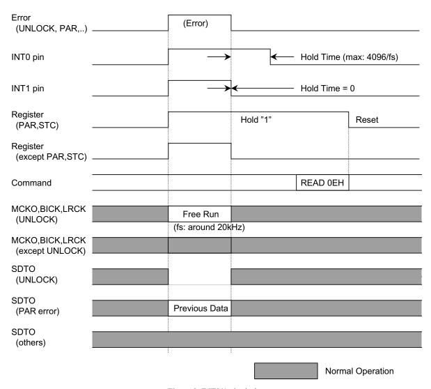
Figure 9. INT0/1 pin timing
