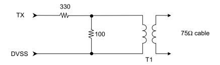
Figure 8. TX External Resistor Network
