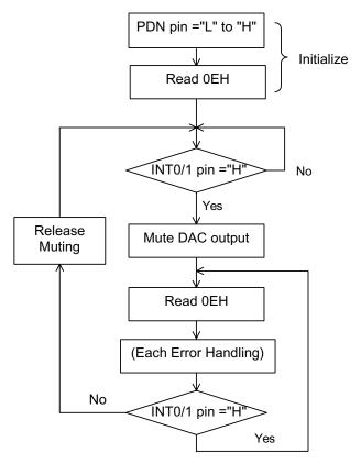
Figure 10. Error Handling Sequence Example
