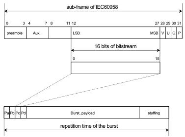
Figure 31. Data structure in IEC60958
