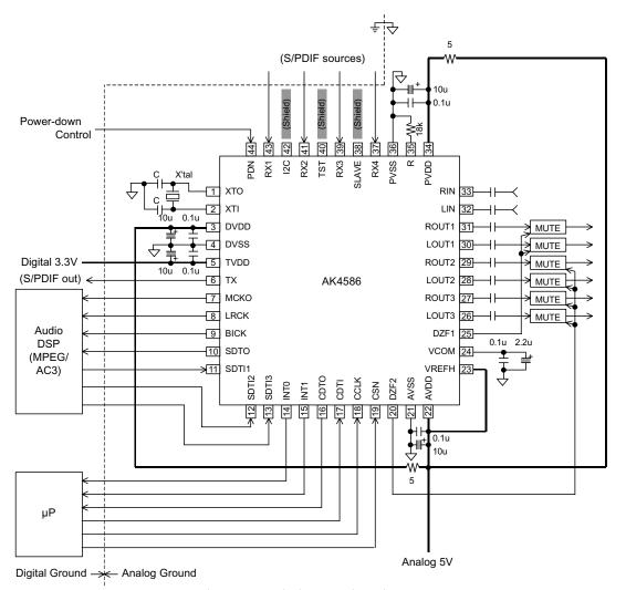
Figure 34. Typical Connection Diagram
