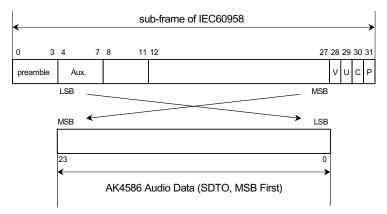
Figure 11. Bit configuration
