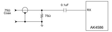
Figure 6. Consumer Input Circuit (Coaxial Input)
