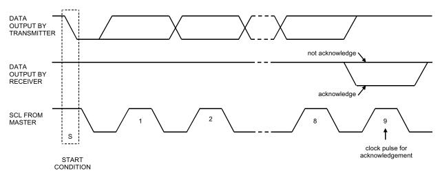
Figure 29. Acknowledge on the I<sup>2</sup>C-bus
