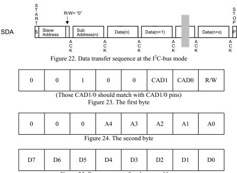
Figure 25. Byte structure after the second byte
