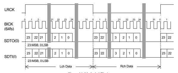
Figure 14. Mode 4, 6 Timing Mode 4: LRCK, BICK: Output Mode 6: LRCK, BICK: Input
