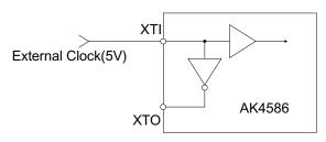
Figure 3. External clock mode(5V) Note: Input clock must not exceed DVDD.
