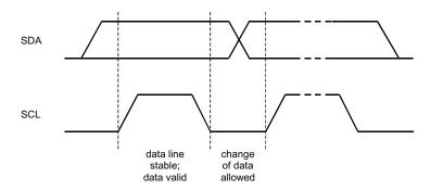
Figure 30. Bit transfer on the I<sup>2</sup>C-bus
