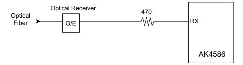
Figure 7. Consumer Input Circuit (Optical Input)
