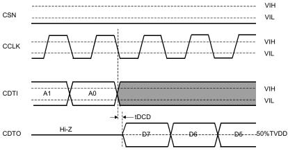
READ Data Output Timing 1 (4-wire serial mode)
