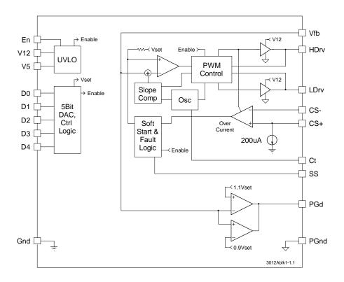
Figure 1 - Simplified block diagram of the US3012/3012A.
